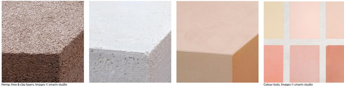
Materially, the core is made from hemp shiv, a waste product from the hemp fibre industry, and hydrated lime. The outer layer is a fibrous lime plaster, coloured with clay. Both hemp and lime are incredibly hard-wearing and resilient, naturally derived materials, and both are also considered to be carbon negative as they capture more carbon than it takes to produce and transport them.
